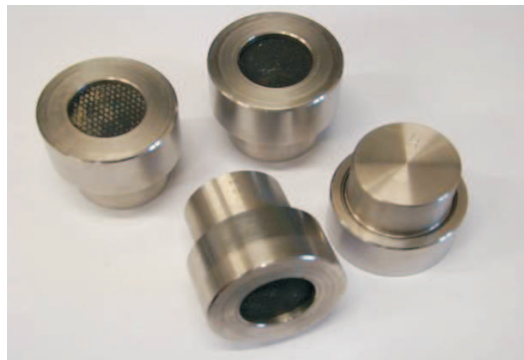
Figure 2. Cells for testing of rubber linings in autoclave.
