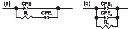
Figure 4. Electric equivalent circuits used in the analysis. CPE, CPE 1 , CPE 2 – Constant Phase Elements, R 1 – resistance.
