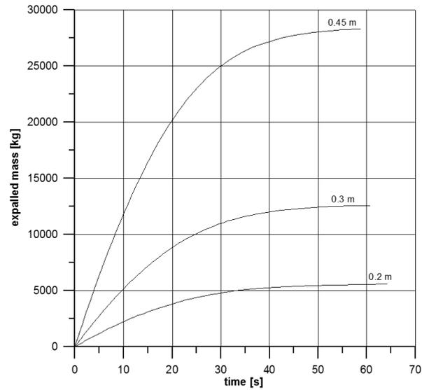
Figure 10. The change in the amount of gas released from part A of the gas pipeline depending on time.
