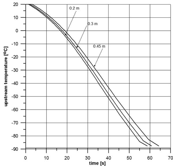
Figure 4. The change in the CO<sub>2</sub> temperature in the damaged pipeline depending on time.
