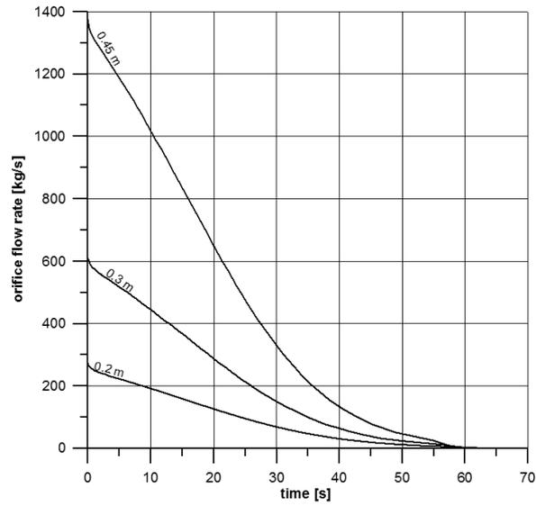
Figure 6. The change in the CO<sub>2</sub> mass flux in the orifice depending on time.
