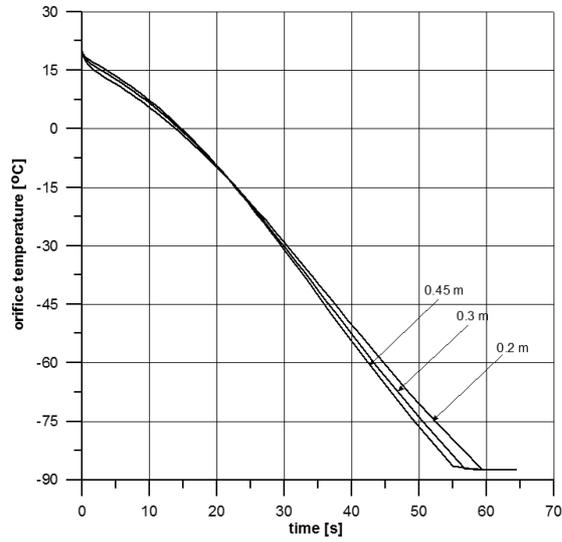
Figure 7. The change in the CO<sub>2</sub> temperature in the orifice depending on time.
