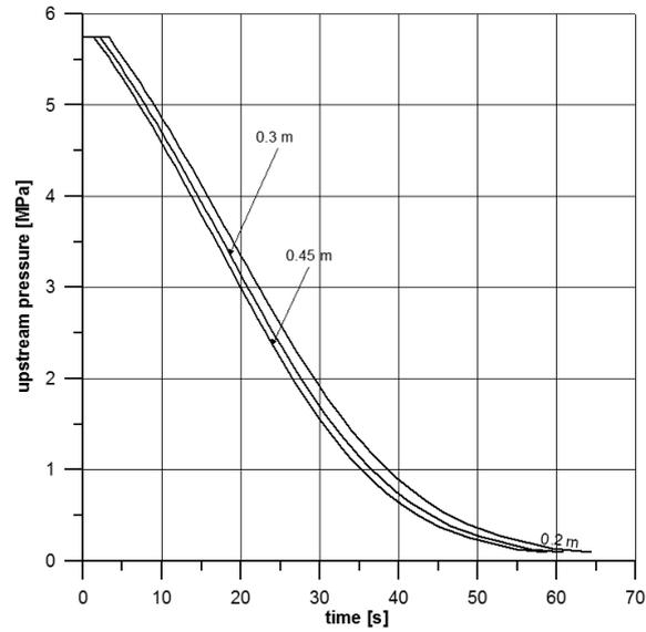
Figure 3. The change in the CO<sub>2</sub> pressure in the damaged pipeline depending on time.
