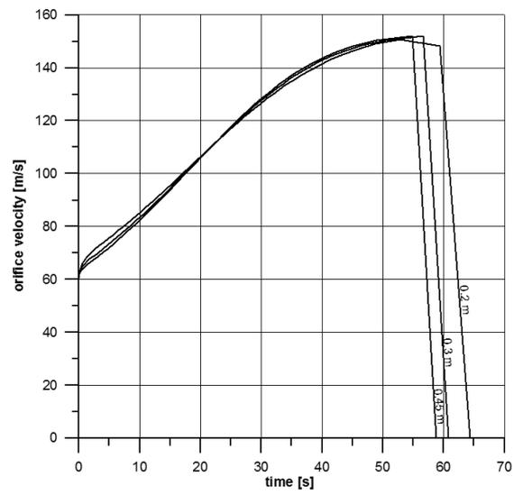
Figure 9. The change in the CO<sub>2</sub> outflow velocity in the orifice depending on time.
