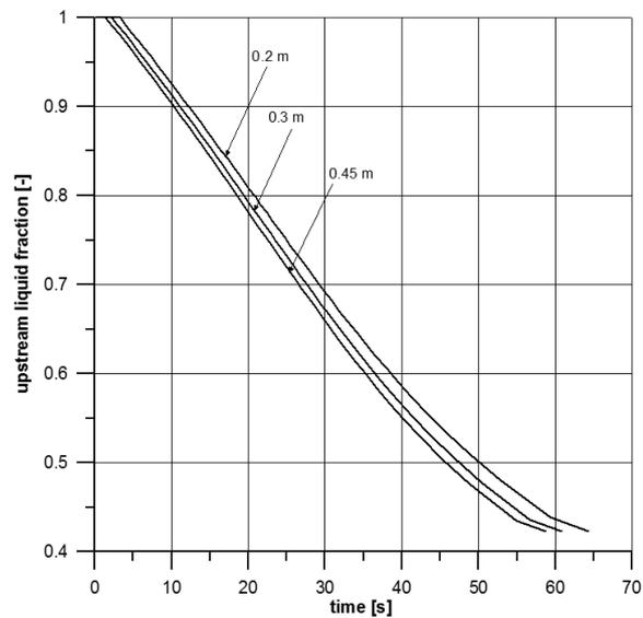
Figure 5. The change in the content of the CO<sub>2</sub> liquid phase in the damaged pipeline depending on time.
