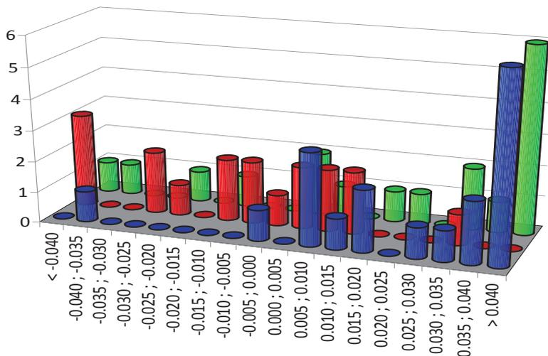
Fig. 9. Histogram of measured frequency for differences in coordinates between RTX-3rd class CAT. methods
