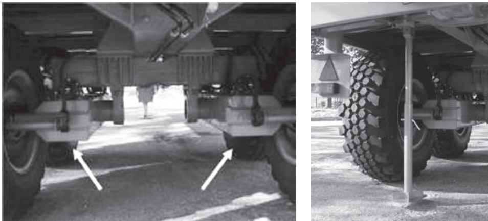
Picture 2. The implemented trailer suspension
