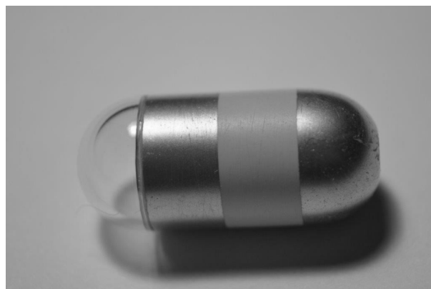
Fig. 1. MicroCam endoscopic capsule measuring 24x11 mm.
