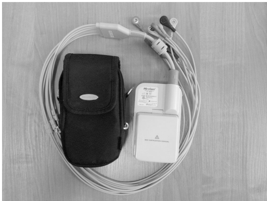
Fig. 2. Data recorder with a battery and electrodes.
