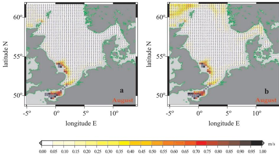
**Figure 12.** (a) Monthly mean of the Ekman flow at 5 m depth for August 1991 [ $\text{m s}^{-1}$ ], (b) difference of the monthly mean of the total flow and the Ekman part at 5 m depth for August 1991 [ $\text{cm s}^{-1}$ ]
