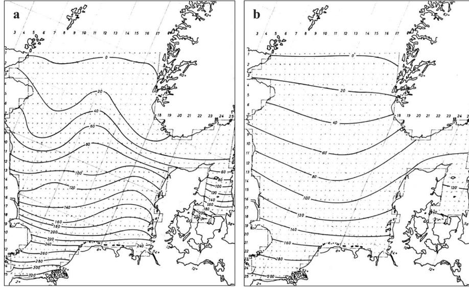
**Figure 3.** Stationary sea level [cm] for a constant northerly wind of  $23.2 \text{ m s}^{-1}$ ; (a) real depth (see Figure 1), (b) constant depth 80 m. From Sündermann (1966)
